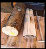
In southern Tasmania, the Huon Wood Centre is a good example of how 21st century timber processing technology is gearing up to maximise the value of wood from regrowth forests and plantations – the main valueadding operations carried out here, such as rotary peel veneer sheet, use only wood from these two sources.
